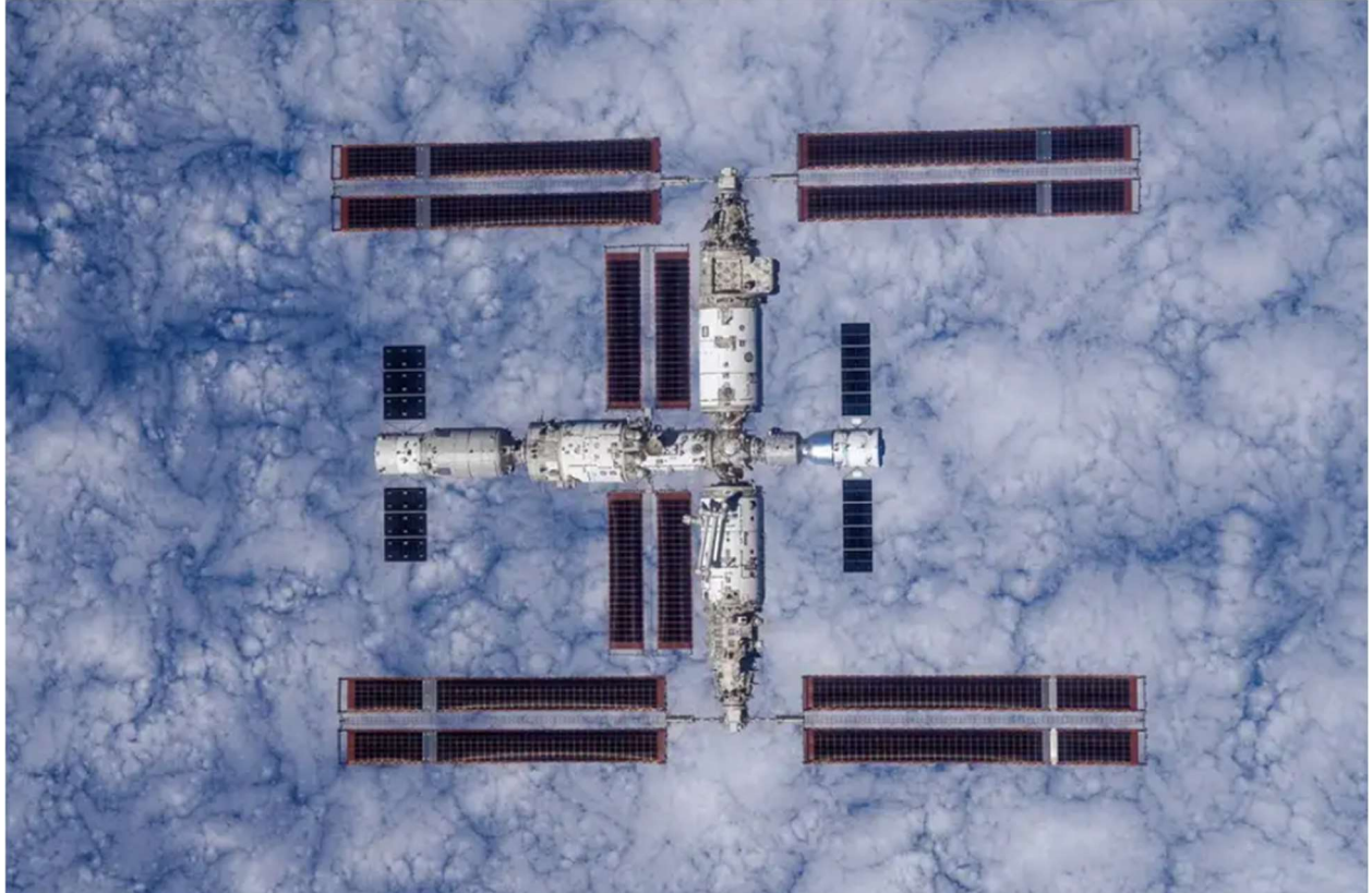
China’s Tiangong space station, photographed from a Shenzhou spacecraft. The Tianhe module, at the center, contains astronauts’ living quarters and a docking hub. The Mengtian module, at the top of the image, and Wentian, at the bottom, are both laboratory modules. Image credit: CMSA
