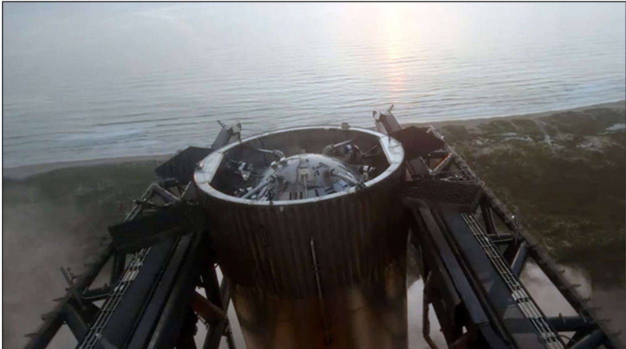
The top of the Super Heavy seen resting between the two mechanical arms at the launch site after its nearly seven minute flight and return “catch” Photo: SpaceX
