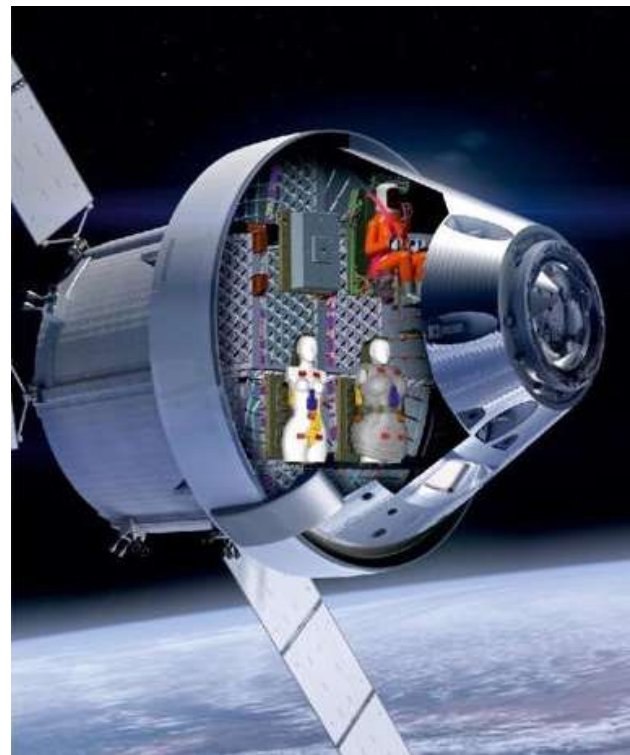
Helga and Zohar on the flight deck of the Orion spacecraft (NASA test mannequin in orange) Credit: Nature (2024). DOI: 10.1038/s41586-024-07927-7
