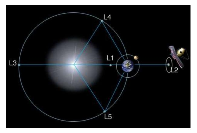
Five locations discovered by mathematician Joseph Lagrange where the gravitational forces of the Sun and Earth (or other large body) and the orbital motion of the spacecraft are balanced, allowing the spacecraft to hover or orbit around the point with minimal expenditure of energy. The L2 point (location of the Euclide and James Webb telescope) is situated 1.5 million kilometers beyond the Earth (as viewed from the Sun).
