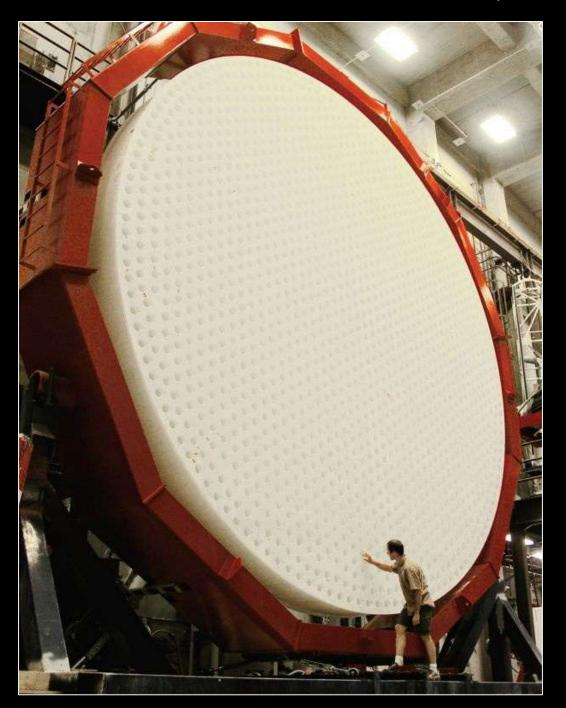
The back surface of one of the seven mirrors cast for the Giant Magellan Telescope. Each 8.4 meter (27.5 foot) mirror is formed from nearly 20 tons of pure optical glass in a rotating furnace at the University of Arizona's Richard F. Caris Mirror Lab located beneath the football stadium. Photo: Ray Bertram/UA
