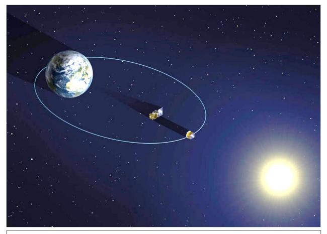
The two Proba-3 spacecraft will orbit Earth in an elliptical path with an apogee of nearly 37,300 miles (60,000 km) and a perigee of some 370 miles (600 km) – (NOT TO SCALE)
