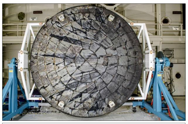
The thermal shield from NASA's Orion spacecraft. The 16.5 feet in diameter (5 meters) shield was removed from the spacecraft at the conclusion of the Artemis I test flight for inspection. Credit: NASA
