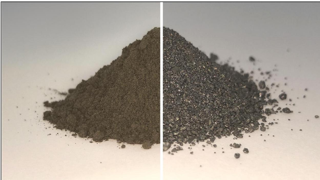
Before and after images of a sample of simulated lunar soil regolith in which essentially all the oxygen has been removed. The end product (right) is a mixture of metallic compounds.
