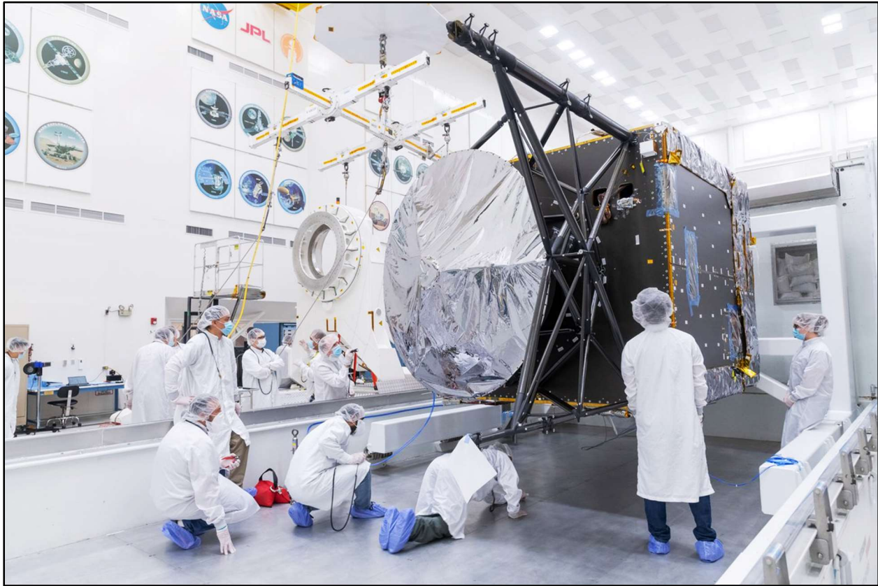
Psyche's SEP Chassis being brought into High Bay 1 of JPL's Spacecraft Assembly Facility Image Credit: NASA/JPL-Caltech
