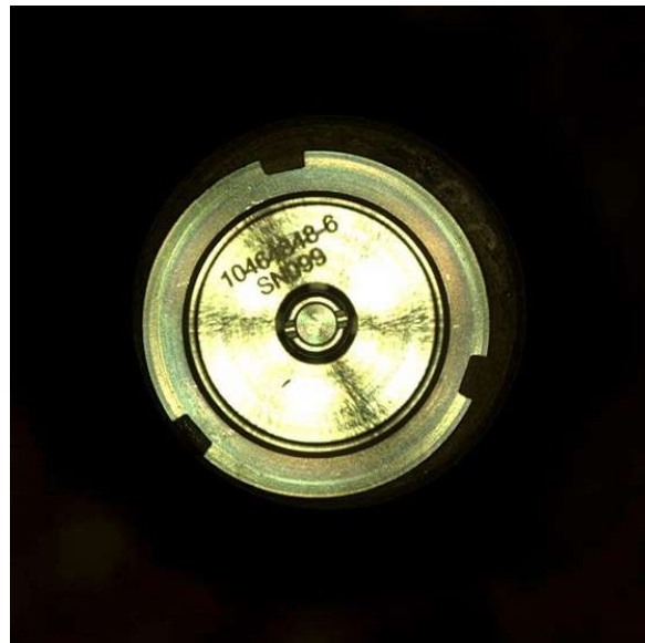
Left: image acquired by the onboard Sample Caching System Camera located inside the rover - looking down the sample tube and at the top of the sampled material Right: the final product - a sealed airtight titanium sample tube, which is then stored inside the rover Image Credit: NASA/JPL-Caltech
