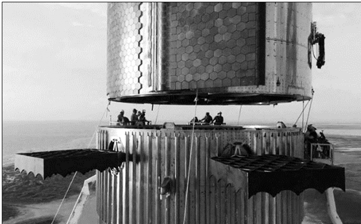
Mating of the Starship (Serial No. 20) with the Super Heavy booster during a fit check Image credit: Elon Musk/Twitter
