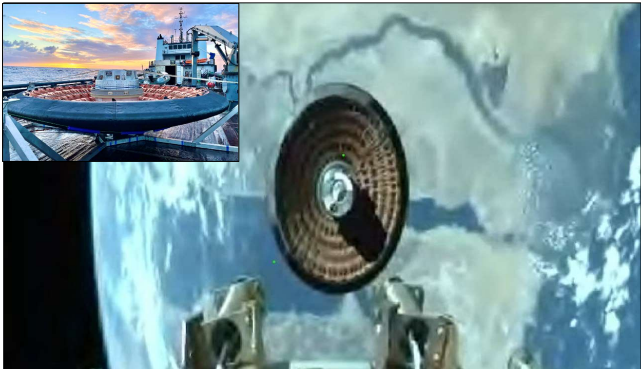
Aft view of LOFTID from the upper stage of Atlas V rocket after deployment and inflation, and subsequent recovery after splashdown (insert) Credit: NASA/Greg Swanson
