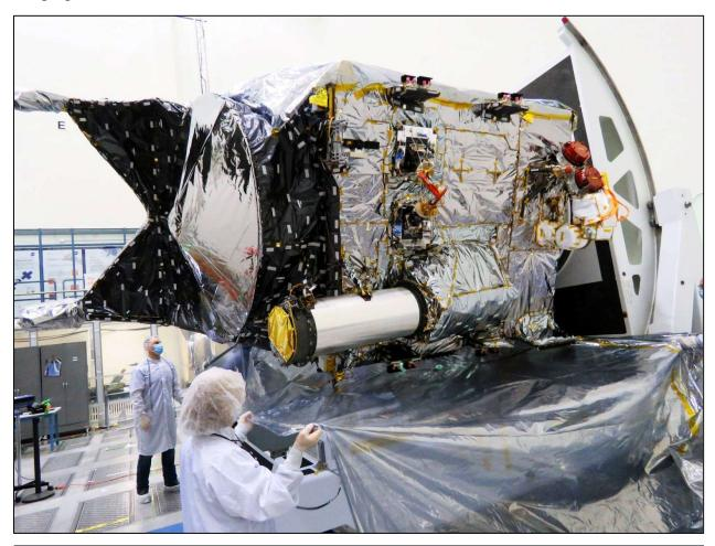
The DSOC flight laser transceiver, distinguished by its prominent tubular sunshade, is mounted on the side of the Psyche spacecraft. The photo was taken during launch preparations. Image credit: NASA/JPL-Caltech
