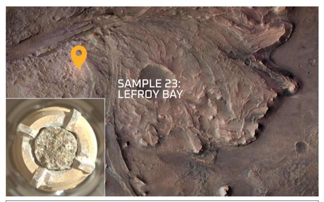
Insert: Core sample No. 23 after being extracted by the rover's rock drill and prior to being transferred into a sample storage tube - imaged by the rover's Left Mastcam-Z camera. Image Credit: NASA/JPL-Caltech/ASU
