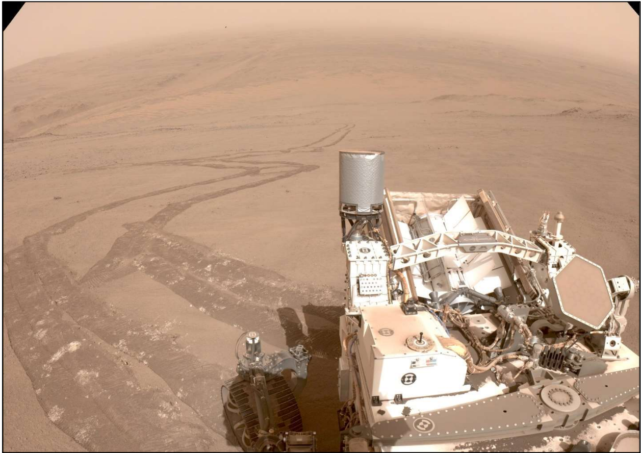
Tracks showing the wheel slippage and surface instability encountered by Perseverance Credit: NASA/JPL-Caltech
