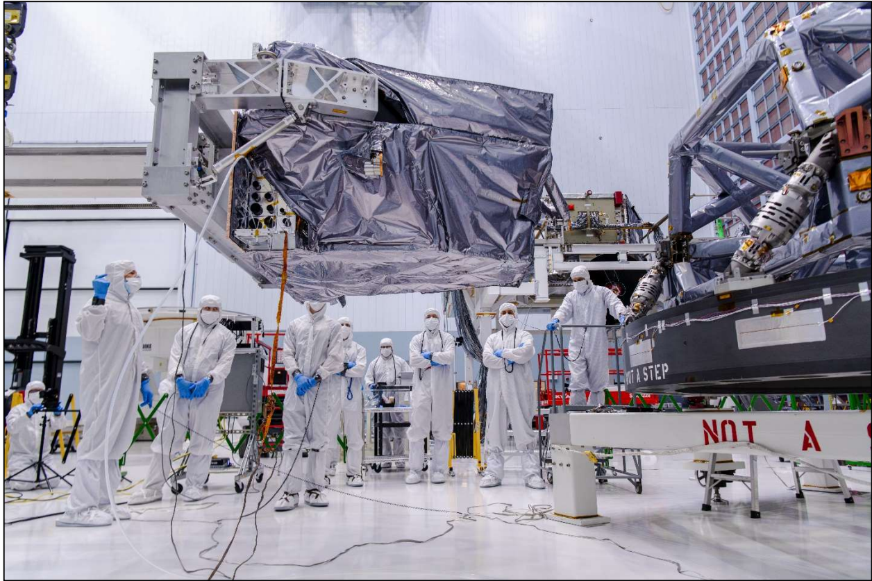
The Roman Coronagraph being installed on the Instrument Carrier at NASA's Goddard Space Flight Center in Greenbelt, Maryland NASA/Sydney Rohde
