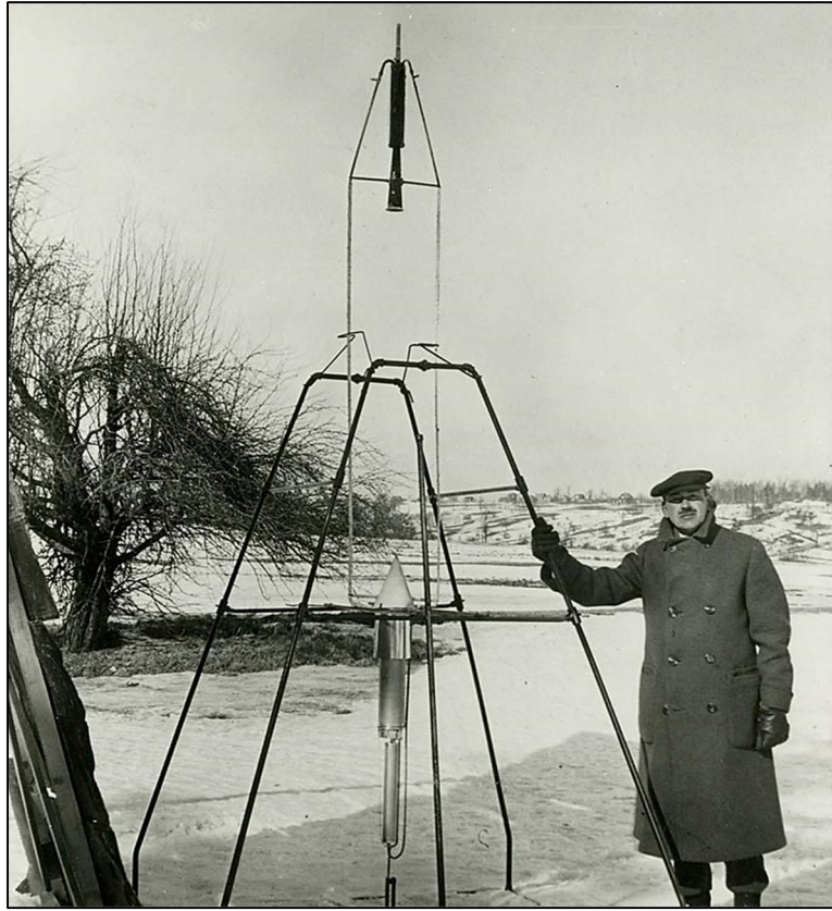
Dr. Goddard with his liquid oxygen-gasoline rocket "Nell" in its launching frame on his aunt's farm in Auburn, MA
